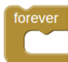
Figure 3: The Google Blockly “forever” block which constantly runs the stack of blocks inside of it.
